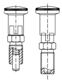
d1 = 5 NV = 12 d2 = M10x1 Spring pressure N bottom = 15.0d3 = 19 Spring pressure N top = 5.0
